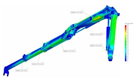
The results of strength calculations performed by a certified authority have confirmed that the ESSEL EC130Z-96 hydraulic crane complies with the STN EN 12999 + A1 standard in terms of strength and fatigue, and also complies with the requirements of the European Parliament Directive 2006/42/EC on machinery. Strength calculations simulate an estimated number of 600,000 duty cycles.
