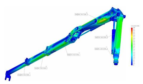
The results of strength calculations performed by a certified authority have confirmed that the ESSEL EC185Z-96 hydraulic crane complies with the STN EN 12999 + A1 standard in terms of strength and fatigue, and also complies with the requirements of the European Parliament Directive 2006/42/EC on machinery. Strength calculations simulate an estimated number of 600,000 duty cycles.
