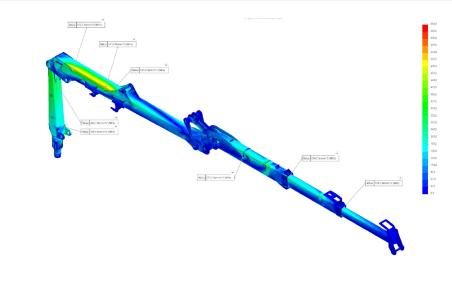
The results of strength calculations performed by a certified authority have confirmed that the ESSEL EC80S-93 hydraulic crane complies with the STN EN 12999 + A1 standard in terms of strength and fatigue, and also complies with the requirements of the European Parliament Directive 2006/42/EC on machinery. Strength calculations simulate an estimated number of 600,000 duty cycles.
